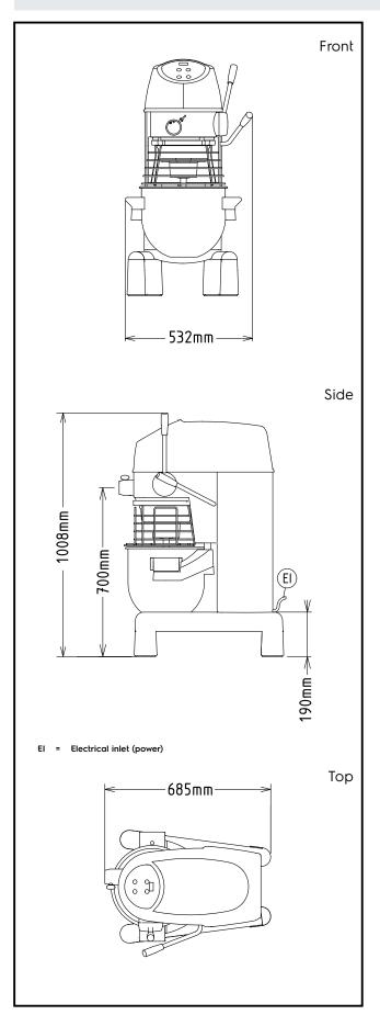
Electric Supply voltage: 600257 (XBM20AT6M) 208-230 V/1N ph/60 Hz Capacity: Performance (up to): ISO 9001; ISO 14001 litres Capacity: **Key Information:**
